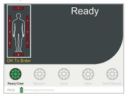
Along with these indicators, a human silhouette, located on the right hand side of the portal frame, indicates which of the eight detector zones are "contaminated" thus aiding in localizing the contamination on an individual. The monitor will utilize double detector and triple detector sum-zones for monitoring of low level distributed activity. Voice commands may be utilized to help with the positioning of the user.
